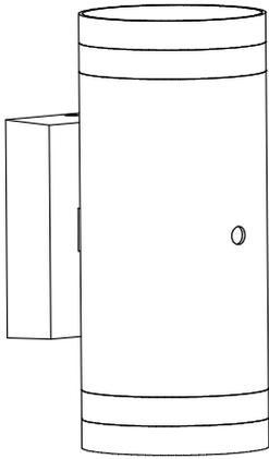
The Dusk till Dawn sensor will operate when the ambient light drops below 20 lux (dusk), and will switch off when the ambient light reaches 80 lux (dawn).
