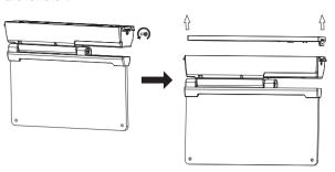
• Click the new bottom plate onto the luminaire main body securely.
